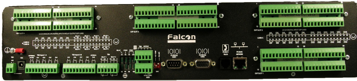
Figure 1.2 FMS Terminal Block Designations
