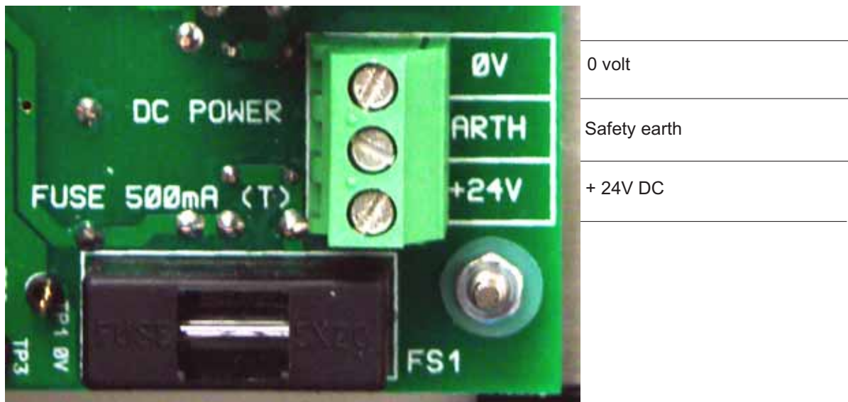
Figure 2-9. Command Module Power Supply Connections
